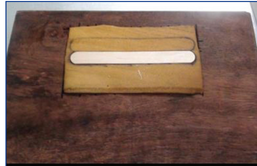
Figure 3. Slot for spatula is cut into the foam.
