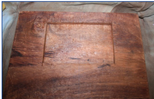
Figure 1. Start with wooden board and cut slot.
